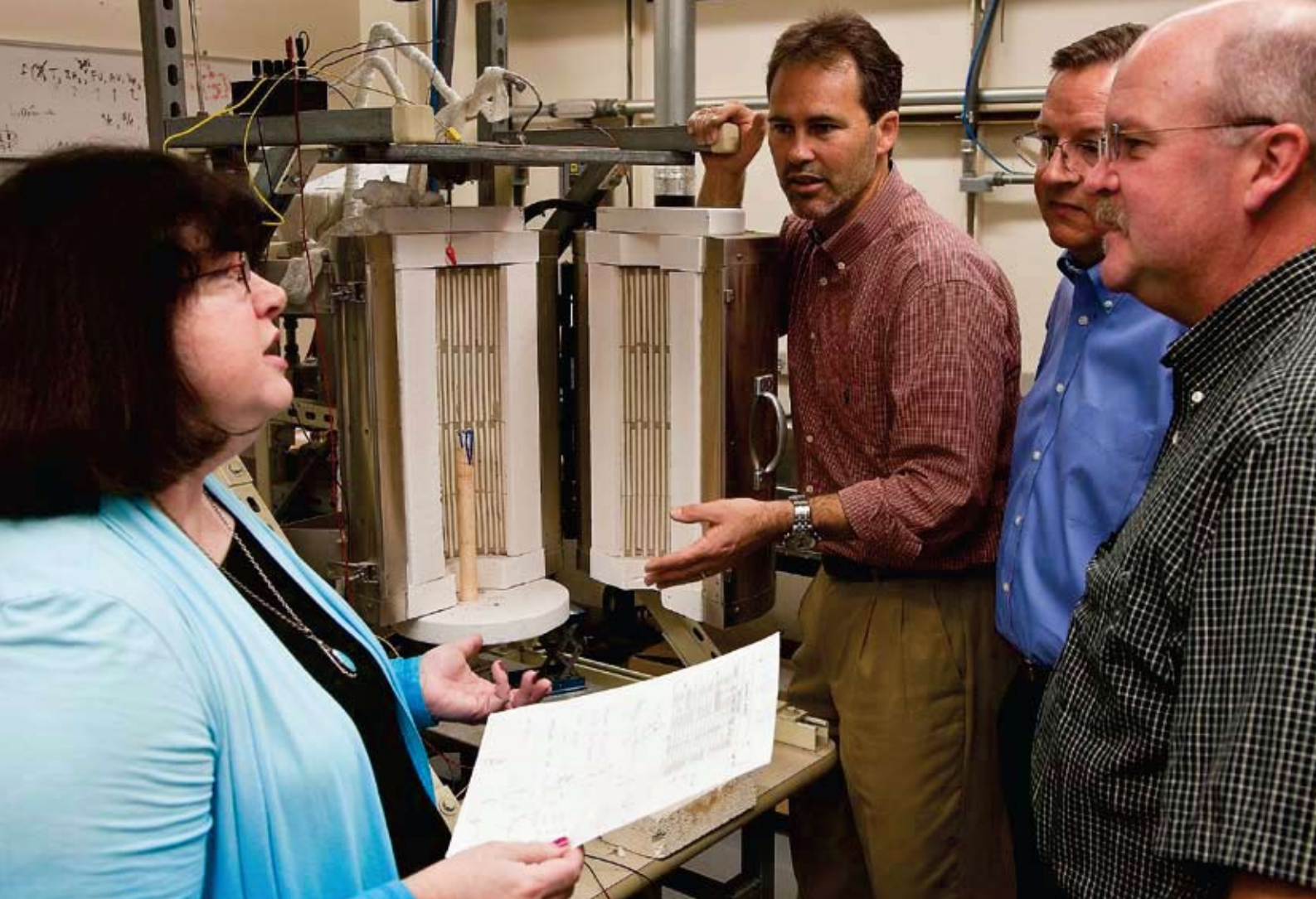
Martha Mecartney discusses a fuel-cell test with (from left) Jack Brouwer, Daniel Mumm and Vince McDonell. The high-temperature furnace in the National Fuel Cell Research Center offers dual-environment controls for testing the SOFC and the solid oxide electrolyzer simultaneously.
